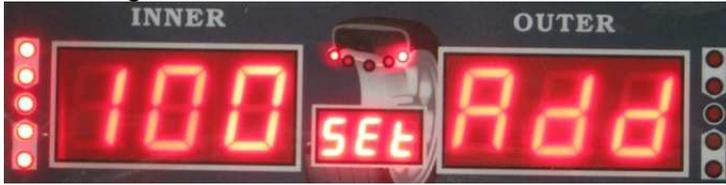
Then place the 100gram or 3.5 Ounce weight that came with the machine at 12 0'clock on the inside of the rim using the provided wheel hammer. 100 grams = 3.5 ounces so either weight is ok. Remember that at anytime you can switch from Grams to Ounces and back by just pushing the **C** button.
