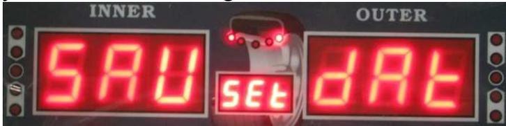
After showing this screen, the machine will automatically return to the initial balancing screen. You have successfully calibrated the machine and the data was saved automatically.
