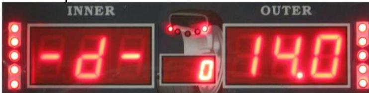
This parameter measures the rim size. This is the D parameter. Use the plastic caliper provided with the machine to measure the width of the rim. Touch the caliper to the edge of the rim on one side to measure the rim size. Use the **UP** or **DOWN** key to enter the parameter. Do not multiply this number like you did with parameter A. Simply enter the number as shown on the caliper.
