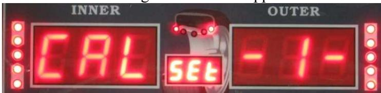
Now push and hold the **ENTER** button. While pushing and holding the **ENTER** button, push and hold the **FINE** button. The following screen will appear:
