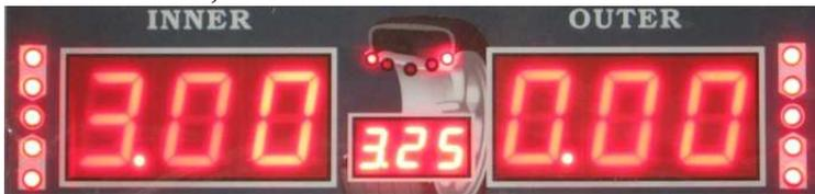
Now place the 3.00 Ounce weight that came with the machine at 12 0'clock on the outside of the rim using the provided wheel hammer. After placing the weight, close the hood and spin the wheel. The following screen will appear:
