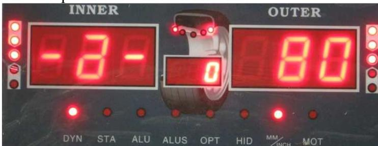
This parameter measures the distance of the wheel from the balancer. This is the **A** parameter. Use the built in ruler and extend it to the edge of the rim. You then multiply the measurement by 10 and enter that number for this parameter using the **UP** or **DOWN** key. For example if the ruler shows 8, you multiply this by 10 to get 80. Enter 80 as
